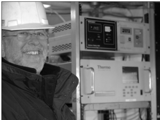
Jerry Slucher is observing NO x , CO and VOC measurements inside the testing trailer at an electric generating facility. DAQ photo
